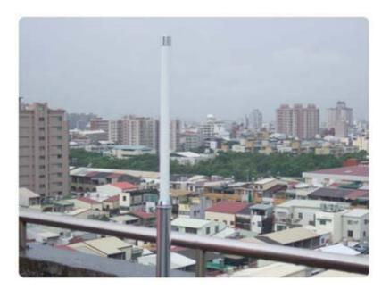
**Photo 3**: Take the antenna to the most remote end of the floor as to receive more WIFI signals. **Photo 4**
